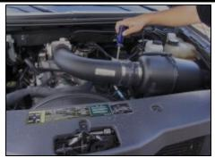
8. Tighten hose clamps on both ends of the Modular Intake Tube.
