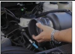
5. Install the supplied silicone hump hose and two #72 hose clamps on factory air filter assembly. Leave hose clamps loose until final assembly.
