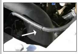
**8.** Spread the supplied hose mount over the radiator overflow hose and push into the hole in the MIT.
