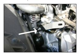
3. Remove 13mm nut on power steering reservoir bracket. Install Airaid Modular Intake Tube support bracket, replace nut, and leave slightly loose. (Nut will be tightened after final adjustments.)
