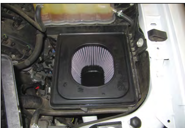
4. Install The Airaid Premium Filter (#1) into the airbox.
