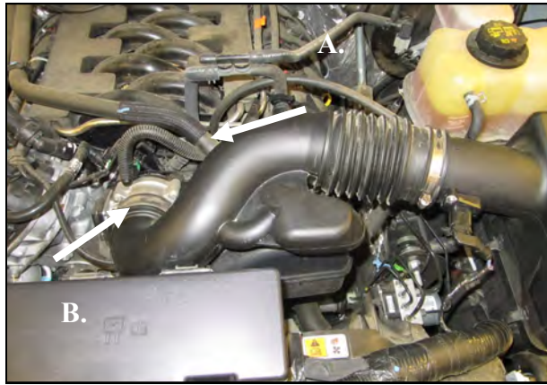
2. A. Disconnect the two breather lines in the factory intake tube. B. Loosen the two intake clamps, and remove the factory intake tube.
