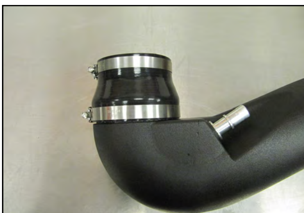
8. Install the Silicone Reducer (#4) and Hose clamps onto the Airaid Intake Tube. Place the #56 Clamp (#18) on the throttle body side of the Reducer, and the #64 Clamp (#9) on to the Tube side.
