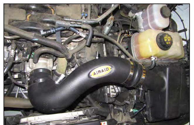
9. Install the Intake Tube onto the throttle body first, then into the airbox. Tighten all of the Hose Clamps.
