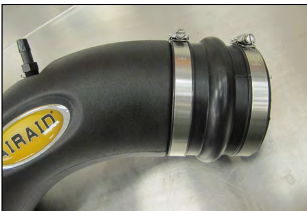
7. Install the hump hose (#3) and two #60 hose clamps (#9) onto the Intake Tube as shown. Leave the hose Clamps loose for now.
