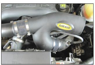
**4.** On late model vehicles, Install the  $1/4^{27}$  Plug into the Airaid Intake Tube as shown. On 2011 models with the vacuum line in the intake, in-
