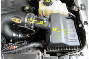
8. Slide the Hump Hose onto the Airaid Intake tube as far as it will go then insert the air box lid tabs into the slots. Adjust the assembly until the lower air box clips can positively engage the lid and lock.
