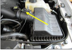
2. Disconnect the wiring harness from air sensor in the air box lid. Unclip the air box lid and remove it and the factory air filter from the vehicle. The lower half of the factory air box is to remain in the vehicle.
