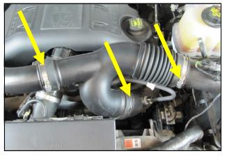
1. Disconnect The Negative Battery Terminal. Loosen the 3 clamps on the factory intake tube and remove it from the vehicle. NOTE: 2011 models will have a vacuum line attached to
