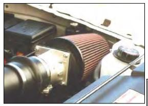
**16.** Install the Airaid Premium Filter (#1) onto the MAF bracket, and tighten the clamp. Reinstall the beauty cover using the three factory bolts.
