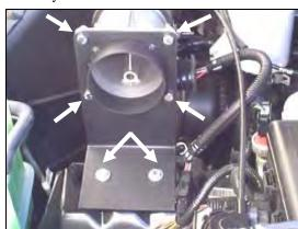
**8.** Mount the **MAF** sensor to the MAF bracket (#3) using four 1/4-20x 7/8" hex bolts (#8), 1/4-20" nylock nuts (#10), and the MAF gasket (#11). Mount the bracket and sensor to the factory location, using the MAF backing plate (#12), two 1/4-20x 7/8" hex bolts (#8), four 1/4" flat washers (#9), and two 1/4- 20" nylock nuts (#10). (Leave the MAF bracket loose for now).
