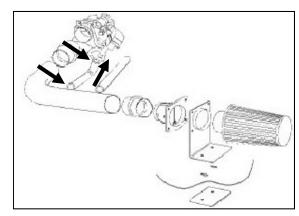
**15.** <u>4.6L engines continued</u>: Connect the Airaid Intake Tube nipple to the IABV inlet tube using the  $3/4 \times 1/2$ " L-hose (#7), and two #22 speed clamps (#17).
