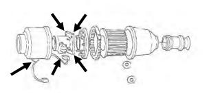
7. Using a 10mm socket, remove the four MAF sensor mounting nuts. Carefully remove the MAF sensor and the wiring harness from the airbox, (save them for reuse).
