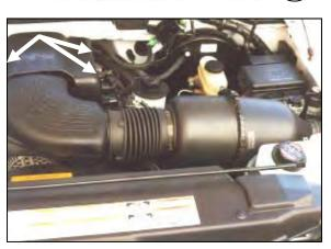
**1.** <u>Disconnect the negative battery cable.</u> Using a 10mm socket, remove the three bolts securing the engine beauty cover, remove the cover, and set it aside (save the bolts and cover for reuse).
