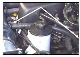
**12.** Install the 5/8"X18" breather hose (#6) onto the valve cover breather fitting then onto the Airaid Intake Tube nipple. Secure the hose using two #19 speed clamps (#16).
