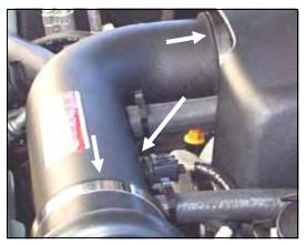
**11.** Install the 7/16" rubber grommet (#15) into the Airaid Intake Tube (#2). Insert the factory **AIT** sensor into the grommet. Slip the Airaid Intake Tube into the urethane hump and reducer hoses. Align for best fit and tighten the remaining hose clamps. Tighten the MAF bracket and reconnect the **AIT** sensor wiring harness.
