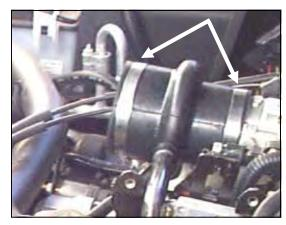
**10.** Install the small side of the urethane reducer hose (#5) onto the throttle body using one #52 hose clamp (#14). Install one #60 hose clamp (#13) onto the larger side of the reducer hose. Tighten only the clamp on the throttle body.
