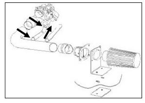
**15.** <u>4.6L engines continued</u>: Connect the Airaid Intake Tube nipple to the *IABV* inlet tube using the  $3/4 \ge 1/2$ ° L-hose (#7), and two #22 speed clamps (#17).
