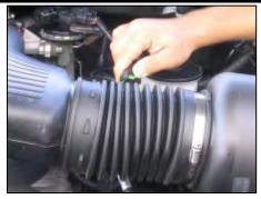
1. Disconnect negative battery cable. Disconnect valve cover breather hose from factory intake tube and valve cover.
