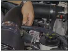
9. Install the supplied rubber hose on the Modular Intake Tube. Connect the other end of the hose to the valve cover. Secure both ends of the hose with the supplied speed clamps.
