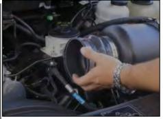
5. Install the supplied urethane hump hose and two #80 hose clamps on factory air filter assembly. Leave hose clamps loose until final assembly.
