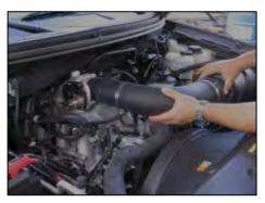
**7.** Install the Airaid Modular Intake Tube on engine.
