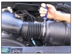
2. Loosen hose clamps connecting the factory intake tube to the air filter assembly and throttle body.
