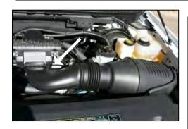
1. Disconnect negative battery cable. Disconnect intake tube from air filter housing by unsnapping the tube assembly from the housing.
