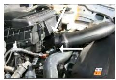
**5.** Install the top of the Airaid MIT into the stock airbox pushing down and in. (*It will snap into place*.)
