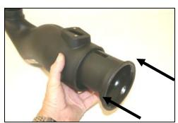
12. Install the Modular Venturi Tube (MVT) (#3) into the Airaid Intake Tube (#2) as shown. Option: For additional air flow, delete the MVT. This requires custom computer programming. Engine damage will result without the use of custom tuning. (SEE #22 BELOW!!)
