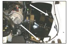
**9.** Install the **CAD** into the factory grommets in the inner fender, and re-install the bolts from steps #3 and #6.
