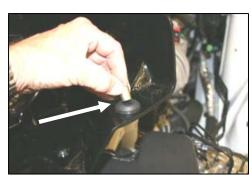
7. Install the provided grommet (#16), with the groove at the top, into the Cool Air Dam (CAD) hole, as shown. Next slide the aluminum sleeve (#17), into the center of the grommet.
