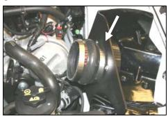
**10.** Install the hump hose (#5) on the filter adapter (#6), with two #64 hose clamps (#14). Tighten <u>only</u> the clamp next to the **CAD**.
