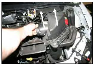
4. Pull straight up, and remove the airbox assembly from the vehicle. It is only held in by one grommet at this point.
