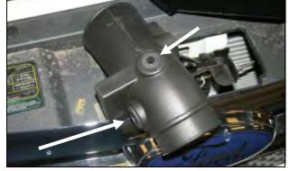
8. Install the small grommet (#20) into the hole on the top of the Airaid intake tube (#2). Now install the large grommet (#21) into the hole on the side of the tube.
