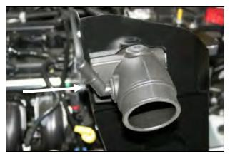
**12.** Insert the factory elbow removed in step #3 into the large grommet on the side of the intake tube as shown. *A drop or two of dish soap or something similar will help make the elbow slide thru the grommet easier.*
