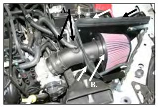
16. A.) Reinstall the small breather hose into the grommet on the top of the intake tube. Reconnect the large breather connector to the factory elbow. B.) Next mount the Airaid Premium Filter (#1) onto the intake tube as shown and tighten the clamp. C.) Install the weatherstrip (#6) onto the top of the CAD panels as shown. Start at the front of the vehicle and work your way towards the fender.
