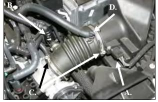
A.) Pull the red tab on the bottom, and then squeeze 2. the Mass Air Flow sensor wiring connector and disconnect it from the sensor. **B.**) Push the tab, and disconnect the breather hose from the plastic elbow. C.) Loosen the two factory clamps on the flexible intake tube. **D.**) Remove the Oetiker clamp, and then carefully remove the small plastic elbow from the flexible intake tube leaving the breather hose connected to the elbow.
