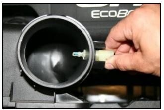
9. Remove the Air Temperature Sensor from the factory air box by rotating the sensor 1/4 turn counter clockwise and pulling outward.
