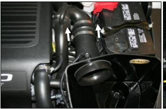
11. A.) Place the CAB in the original location of the 12.Install the Airaid Premium Filter (#1) onto the Filter Factory Air box and secure using the factory hardware adapter and tighten the clamp. from step 4. B.) Slide the coupler and clamps onto 90 deg. Elbow pipe and tighten the clamps. C.) Reconnect the Air Temperature Sensor.
