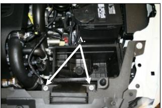
**4. A.)** Using an 8mm socket, remove the two factory **5.** Remove the factory air box assembly from the vehicle. air box bolts and set aside. The will be reused in step 11. **B.)** Remove the factory air filter element.
