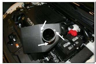
7. Install the Filter Adapter to the inside of the Cool Air 8. A) Install the Hump Hose, large side first (#4) onto Box, CAB (#2) using the three 1/4"-20 hex head bolts the CAB tube. Loosely install the #56 Hose Clamp (#10) (#6) and 1/4" flat washers (#7) as shown.
