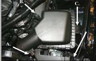
3. A) Slide the red tab, and disconnect the wiring harness from the Mass Air Flow sensor (MAF). Carefully pry the harness anchor from the air box using a screwdriver. B) Separate the resonator tube from the stand off attached to the Air box lid. C) Using a 10mm socket, remove the bolt securing the air box to the inner fender and remove the air box assembly. This bolt will be reused in step 9.
