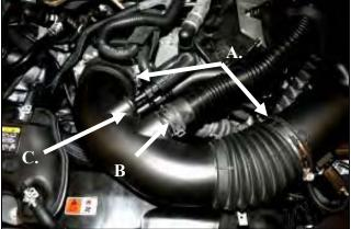
2. A) Loosen the hose clamps on the factory intake tube **B**) Squeeze the clamp and disconnect the resonator from the air intake tube. C) Carefully depress the hose lock tabs, and disconnect the crank case breather line and the brake aspirator line (if equipped, AT models only). D) Remove the factory intake tube.
