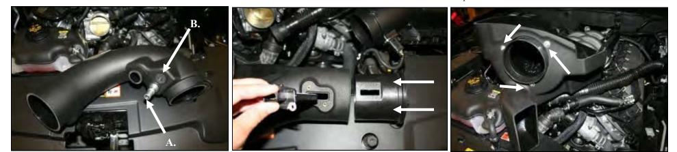
Fitting (#19) and the 5/8"Grommet (#20). B) Automatic bly. transmission equipped vehicles will also use the 3/8" Fit- A) Slide the Modular Venturi Tube (#3) into the ting (#18) and 3/8" Grommet (#21). Manual transmission vehicles will not need the 3/8" components and will use the Blind Grommet(#22).
