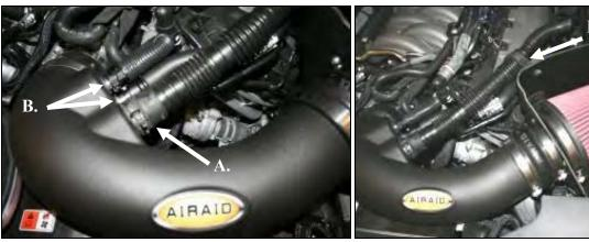
11. Install the Airaid Intake Tube into the couplers as 12. A) Install the Airaid Premium Filter (#1) onto the Resonator tube to the Airaid Intake using the OEM Resonator tubing into the factory Stand off. clamp. B) Reconnect the breather line/lines to the Aluminum Fittings depending on your application.
