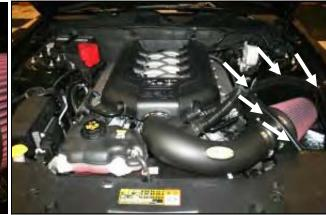
13. Reconnect the Mass Air Flow sensor, which is now 14. Install the Weather Strip (#9) onto the CAB with the located in the lower back side of the intake. Slide the contoured edge going away from the filter. Start at the front of the vehicle and work your way back. Replace the engine cover.
