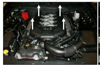
**Disconnect The Negative Battery Terminal!** 1. Remove the strut tower brace, if so equipped. Remove the Engine cover by simply lifting up, and set aside.
