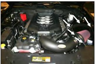
13. Reconnect the Mass Air Flow sensor, which is now 14. Install the Weather Strip (#7) onto the CAB with the contoured edge going away from the filter. Start at the front of the vehicle and work your way back. Replace the engine cover.
