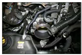
10. Install the Silicone Reducer (#5) and Hose clamps onto the throttle body. Place the #56 clamp (#13) on the Throttle body side of the reducer, and the #64 clamp (#12) on to the tube side.
