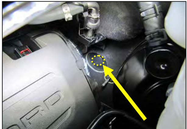
18. Insert the supplied Firewall Plug to prevent debris from entering the cabin as shown.
