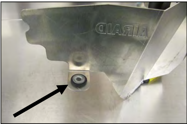
10. Transfer the OEM air box grommet and anti-crush sleeve into the Panel assembly as shown.
