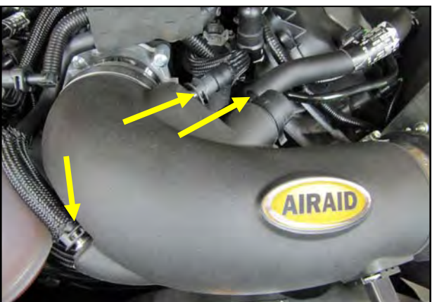
19. Insert the Intake Tube into the Hump Hose and Reducer then tighten all 4 Intake Clamps. Reconnect the factory breather lines.
