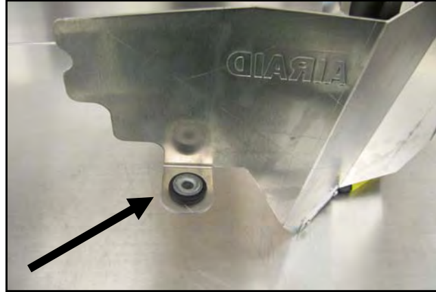
9. Transfer the OEM air box grommet and anti-crush sleeve into the Panel assembly as shown.
