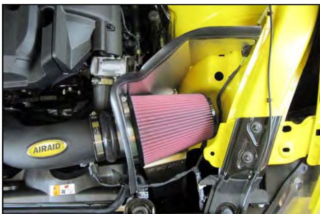
11. Install the Airaid Premium Filter onto the Filter Adapter. Install the weatherstrip on top of the Panel assembly as shown with the contour rolling away from the filter.
