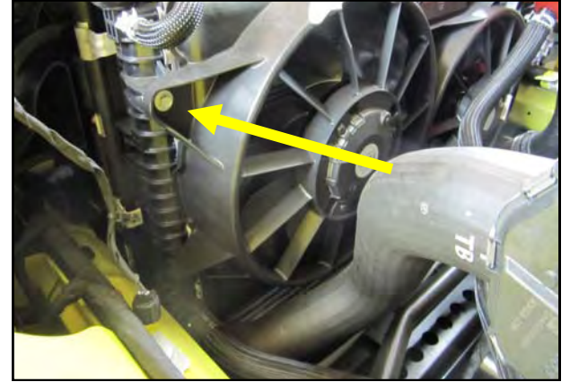
10. Remove the drivers side fan shroud bolt and set it aside.
