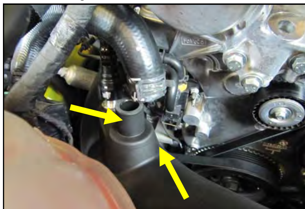
17. Reconnect the PCV and bypass line to the Airaid Intake Tube.
