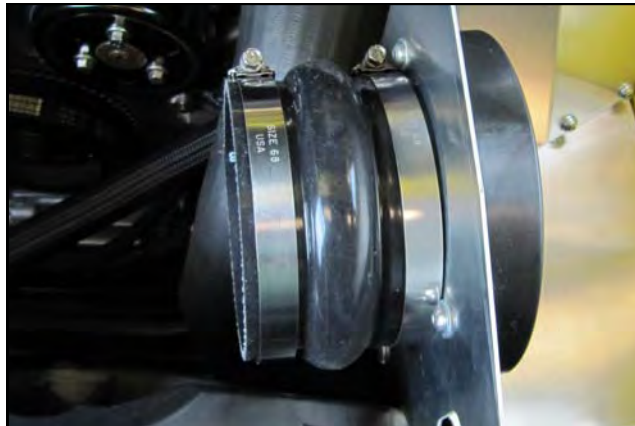
11. Slide the Hump Hose with two, #68 Clamps onto the Filter Adapter .
