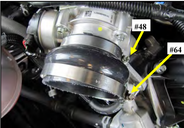
14. Slide the Reducer with one #64 and one #48 clamp onto the throttle body as shown.
