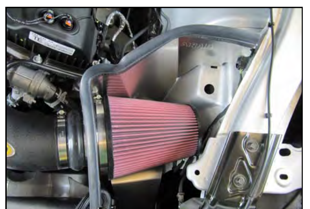
18. Install the weatherstrip on top of the Panel assembly as shown with the contour rolling away from the filter.
