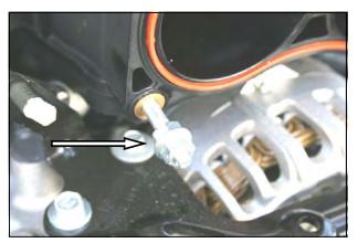
3. Using the two nuts removed in step #2, install them as shown, on one of the studs, snug them together, and then turn the nut closest to the manifold, and remove the stud. Repeat the procedure on the second stud.
