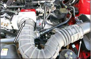
4. Reinstall the intake tube, and tighten the hose clamps.
