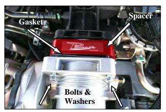
3. Install two bolts (#2), and washers (#3) thru the throttle body, thru the gasket (#4), thru the Poweraid Spacer (#1), and into the intake manifold as shown. Use caution to retain the factory o-ring gasket on the plastic intake manifold.
