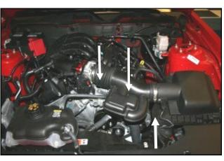
7. Reinstall the intake tube, tighten the two hose clamps, and reconnect the breather line or lines.
