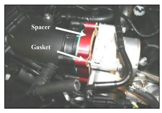
**4.** Position the Poweraid Spacer between the throttlebody and the intake manifold with the supplied gasket next to the throttlebody as shown. Make sure the "flow" arrow that is printed on the spacer is pointing towards the intake manifold. Insert the provided bolts and washers through the throttlebody, gasket, and Poweraid Spacer.
