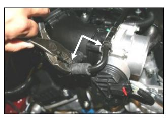
**2.** Using pliers, open the spring clamps and slide off of the factory breather hose, and onto the hard line.
