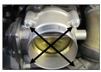
2. Remove the four bolts that secure the throttlebody to the intake manifold and set them aside. They will not be reused.
