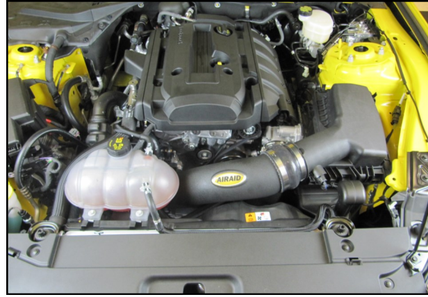
12. Double check your work. Make sure all clamps, hoses, bolts, and screws are tight. Double check the hood clearance. Reconnect the negative battery cable and reinstall the cover.
