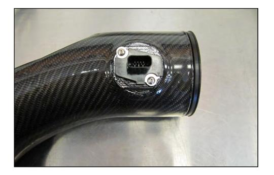
**3.** Transfer the Mass Air Flow sensor from the plastic tube into the Carbon Fiber intake, and re use the  $8-32 \times 3/8$ " screws.
