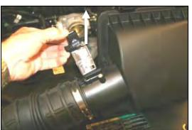
2. Remove bolt that holds the factory airbox to the
