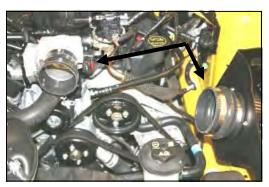
13. Install the urethane hump hose (#4) on the filter adapter (#5) with two #72 hose clamps (#13). Next install the reducing coupler (#3) small end first, onto the throttle body with one #48 hose clamp (#11), and one #52 hose clamp (#12). Leave clamps loose.
