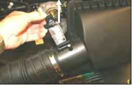
**6.** With a pair of side cutters, remove the metal band that holds the plastic breather fitting in the factory tube. Next remove the fitting from the tube, and save it for reinstallation in step #11.
