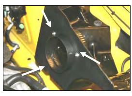
9. Install the filter adapter (#5) into the CAD using three button head bolts (#8), and washers
