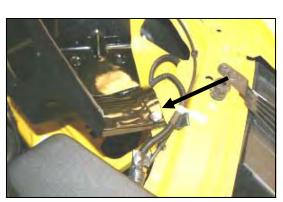
**8.** If your vehicle has the optional anti-lock brakes, remove the bolt from the bracket under the CAD, and reinstall it thru the hole in the front of the CAD. (See arrow). If your vehicle does not have this bracket, install the supplied 1/4" bolt (#14), two 1/4" washers (#9), and 1/4" Nylock nut (#15) thru the CAD and sheet metal, and tighten.
