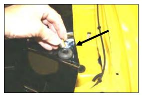
7. Install the tall grommet (#17), (groove at the top), into the Cool Air Dam (#6), and then slide the aluminum sleeve (#18) into the grommet as shown. Install the CAD thru the 2 factory grommets in the fender and reinstall the factory bolt from step #2.
