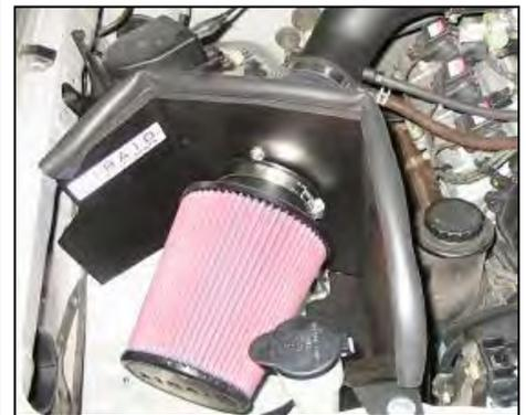
15. Mount the Airaid premium air filter inside the Cool Air Dam & press weather strip onto the top of the Cool Air Dam. (*Hint: start at a corner and work towards the ends*)
