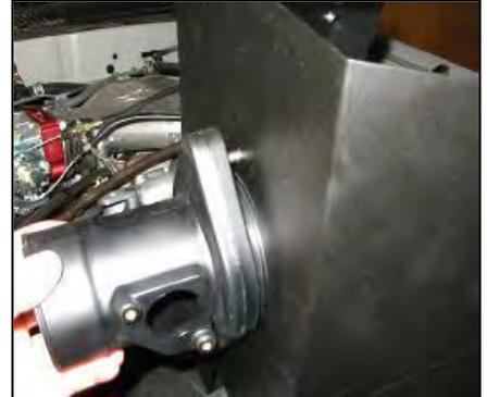
7. Using two supplied 1/4-20 bolts and washers, mount the Airaid filter adapter to the Airaid Cool Air Dam.
