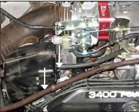
2. Remove factory vacuum lines / hose from the factory air box and intake tube. (*Note: Retain the 3/8" vacuum hose*)
