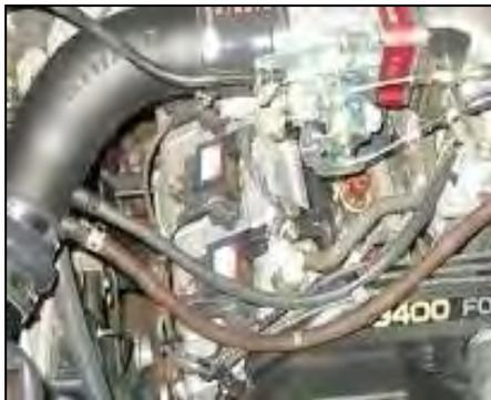
13. Connect factory 3/8" vacuum line to nylon fitting on intake tube & connect steel tube on intake manifold to 1/4" fitting on intake tube with 1/4" vacuum line provided.
