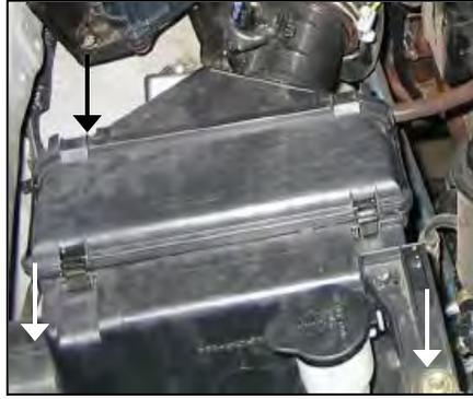
4. With a 12mm socket, remove the three bolts securing the factory air box assembly & remove the factory air box assembly from vehicle.
