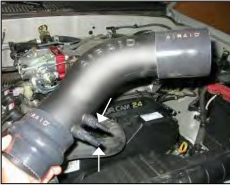
9. Install two supplied 1/4" NPT barbed fittings in Airaid intake tube. (*Note: Install 3/8" fitting in the forward hole and the 1/4" fitting in the back hole*) Slide hump hose and two #52 hose clamps on large end of intake tube and slide coupler with two #48 hose clamps on small end of tube. (*Note: leave all hose clamps loose for final assembly*)
