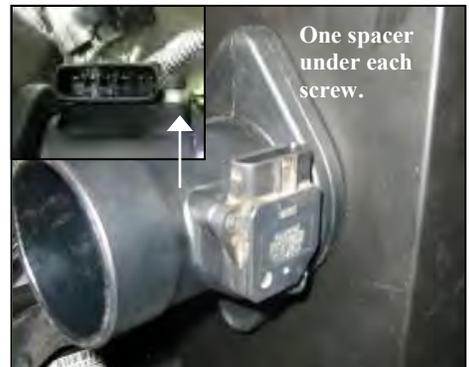
8. Using the two 8-32 Allen head screws and two plastic spacers provided, mount the factory Mass Air Sensor to the Airaid filter adapter tube. (*Note: the plastic spacers are placed between the Mass Air Sensor and the Filter Adapter Tube with the screws sliding through the spacers*).
