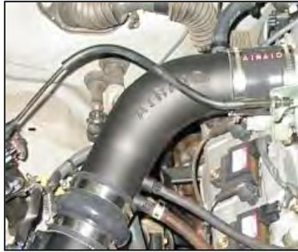
11. Connect the Airaid intake tube to the engine by sliding the coupler over the throttle body & adjust the intake tube to insure proper alignment from the throttle body to the air filter adapter. (*Note: Leave a gap between the tube and the air filter adapter to allow for engine movement*)
