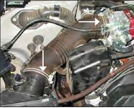
1. Disconnect the negative battery cable, then, loosen the two hose clamps on the factory intake tube.
