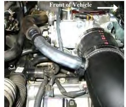
14. Using the supplied 5/8" to 1/2" barbed connector and 1/2" x 4" breather hose, connect the factory hose located by the throttle body to the Airaid intake tube. Use two supplied #16 Speed clamps to secure the hose to the barbed ends.
