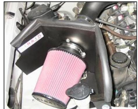
15. Mount the Airaid premium air filter inside the Cool Air Dam & press weather seal onto the top of the Cool Air Dam. (*Hint: start at a corner and work towards the ends*)
