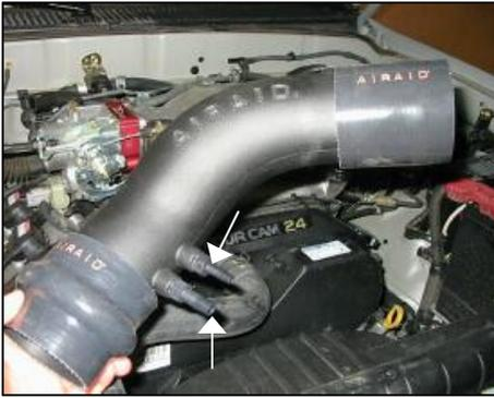
9. Install two supplied 1/4" barbed fittings in AirAid intake tube. (*Note: Install 3/8" fitting in the forward hole and the 1/4" fitting in the back hole*) Slide hump hose and two #48 hose clamps on large end of intake tube and slide coupler with two #44 hose clamps on small end of tube. (*Note: leave all hose clamps loose for final assembly*)
