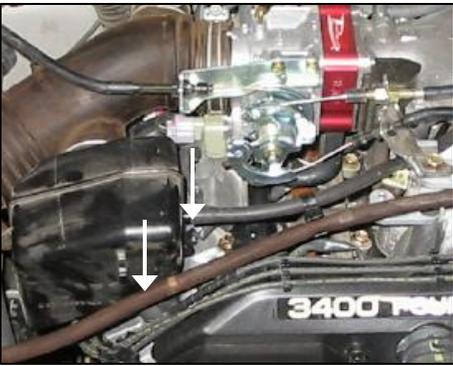
2. Remove factory vacuum lines / hose from the factory air box and intake tube. (*Note: Retain 3/8" vacuum*)
