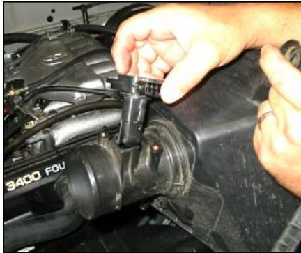
5. Loosen the two screws on the Mass Air Sensor and remove the sensor from the factory air box. Retain sensor for later use.
