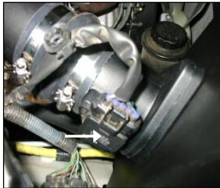
12. Reinstall the electrical connector to the Mass Air Sensor.
