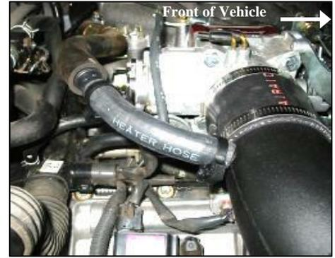
14. Using supplied 5/8" to 1/2" barbed connector and 1/2" x 4" hose; connect the factory hose located by the throttle body to the Airaid intake tube. Use two supplied #16 Snapper clamps to secure the hose to the barbed ends.
