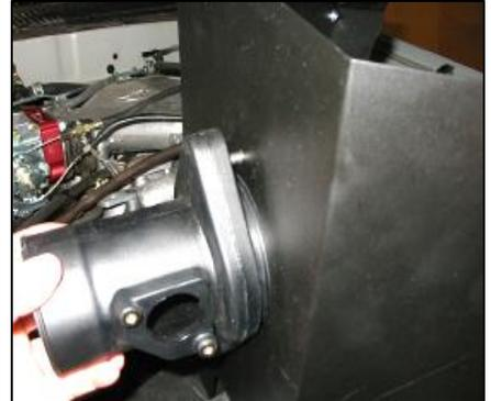
7. Using two supplied 1/4-20 bolts and washers, mount the Airaid filter adaptor to the Airaid Cool Air Dam.
