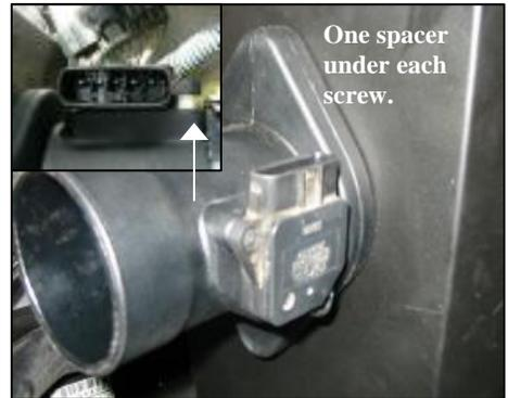
8. Using the two 8/32 Allen head screws and two plastic spacers provided, mount the factory Mass Air Sensor to the Airaid filter adaptor tube. (*Note: the plastic spacers are placed between the Mass Air Sensor and the Filter Adapter Tube with the screws sliding through the spacers.*)
