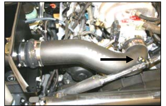
15. Install the Airaid MIT (#5) into the hump hose first, and then into the coupler. Adjust the MIT snugly against the throttle body and tighten the all four clamps. Install the supplied button head bolt (#17), and washer (#18) thru the Adel clamp, and thread into the MIT. (See arrow)
