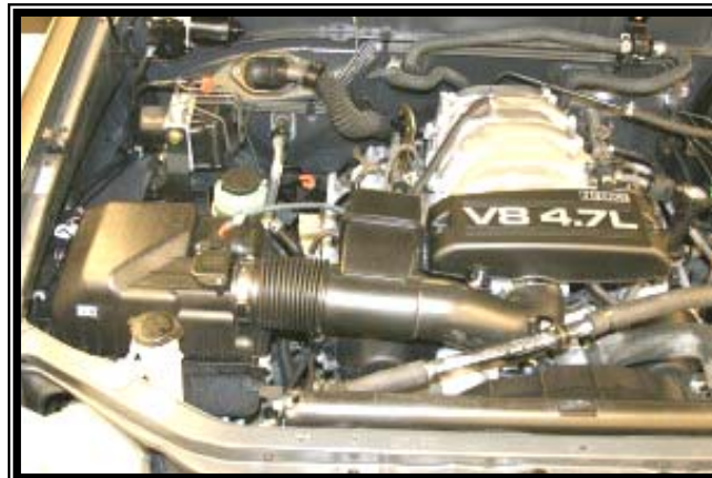
16. A) Install the 1/2"x13" breather hose from the MIT to the valve cover. B) Install the vacuum tee (#12) into the 1/4"x4" hose (#13) and then into the factory 1/4" vacuum hose, and 1/8" vacuum hose as shown. Refer to the hoses in step #11. Reinstall the beauty cover from step #10.
