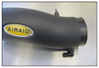
**9.** Install the 1/8" and 3/8" barbed fittings (#s 11 and 12) into the Airaid Intake Tube as shown.
