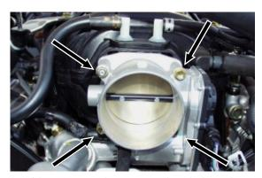
4. With a 10mm socket, remove three bolts and one nut from the throttle body. Slide the throttle body away from the intake manifold, and remove the remaining stud.
