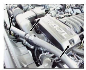
1. <u>Disconnect the negative battery cable!</u> Remove two 10mm nuts that hold the beauty cover to the engine. Set the beauty cover and nuts aside for re-installation later. Loosen the hose clamp that holds the intake tube to the air filter box.
