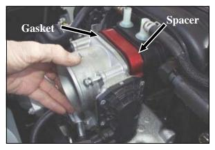
5. Install the Poweraid spacer (#1) next to the intake manifold, and the fiber gasket (#4) next to the throttle body. Insert the four provided 6mm bolts (#2), and washers (#3), and tighten in a cross pattern, to the vehicle manufacture's specifications.
