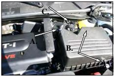
1. Disconnect the negative battery cable! A). Loosen the hose clamp that holds the factory intake tube to the air cleaner lid. B). Loosen the two bolts that hold the lid of the air cleaner to the base. C). Disconnect the wiring harness from the mass air sensor.
