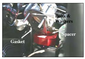
**5.** With the gasket (#4) on top of the Poweraid Spacer (#1), lift the throttle body up, and slide the spacer between the manifold, and the throttle body. Install four 8mm bolts (#2) and washers (#3) thru the throttle body, gasket, spacer, and into the manifold.
