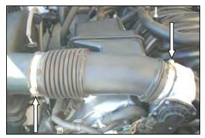
**2.** Using a 10mm socket, loosen two hose clamps on the factory intake tube. Slide the factory intake tube off of the throttle body and airbox. Move the factory intake tube aside, while leaving the factory vacuum and breather lines connected.
