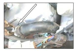
**3.** Using pliers, squeeze the tabs on the coolant hose clamp together. Slide the hose and clamp towards the passenger side approximately one half inch.
