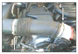
**5.** Re-install the factory intake tube and tighten the hose clamps securely.
