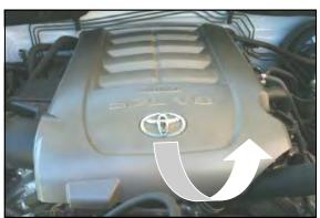
1. Disconnect the negative battery cable! Remove the engine beauty cover by lifting up on the front, and then pulling it towards the front of the vehicle. (Save for reuse).
