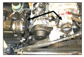
**7.** Install the hump hose (#3) onto the factory airbox, small end first, with two hose clamps (#6). Next install the reducing coupler (#4), small side first, onto the throttle body with two hose clamps (#6). Leave the clamps loose.
