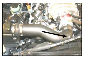
**9.** Install the MIT into the hump hose first, and then into the reducing coupler. Adjust the MIT snugly against the throttle body, and tighten the 4 hose clamps. Next install the supplied button head bolt (#11) and washer (#10) thru the Adel clamp and into the MIT to hold the air conditioning hose.
