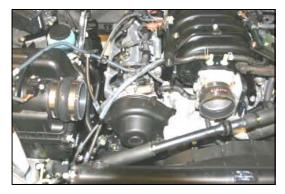
7. Install the hump hose (#3) onto the factory airbox with two hose clamps (#6). Next install the reducing coupler (#4), small side first, onto the throttle body with two hose clamps (#6). Leave the clamps loose.
