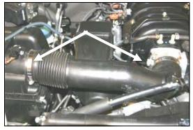
3. Loosen the hose clamps on the intake tube at the throttle body, and at the airbox.
