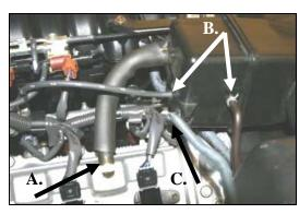
2. A) Disconnect the breather hose at the valve cover. B) Disconnect 1/8" and 1/4" vacuum lines on back of intake tube. C) Unclip wire harness retainer from back of intake tube.
