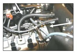
**10.** A) Install the 1/2"x 13" breather hose (#5) from the MIT to the valve cover. B) Install the 1/4"x1/4"x1/8" vacuum tee (#8 into the 1/4"x4" hose (#7) and then to the factory 1/4" and 1/8" vacuum lines, as shown.
