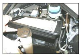
6. Remove the factory air filter, and install the Airaid Premium Filter (#1). Reinstall the factory airbox lid, and latch 4 clips.
