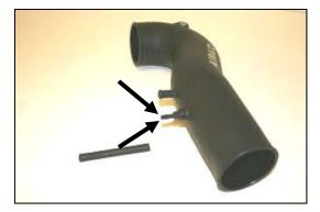
**8.** Install the 1/4" barb fitting (#9) into the Airaid Modular Intake Tube (#2) as shown. Now slide the 1/4"x4" hose (#7) onto the barb fitting.
