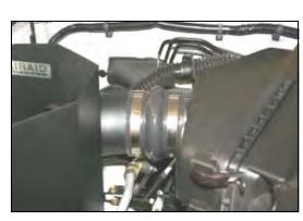
**14.** Center the hump hose between the tube on the factory airbox, and the tube on the **CAD**, adjust for fit, and tighten the hose clamps. Now tighten the button head bolt that holds the bracket to the **CAD**.
