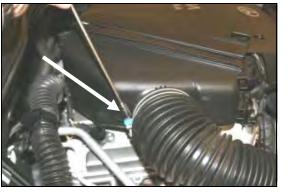
1. <u>Disconnect the negative battery cable.</u> Loosen the hose clamp on the factory intake tube where it connects to the airbox.
