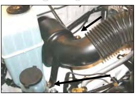
**2.** With a 12mm socket, remove two bolts that hold the intake tube to the fender.
