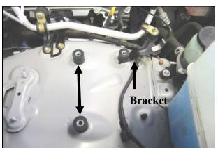
**5.** Install two of the M8 CAB Mounts (#13), hand tight, into the weld nuts on the inner fender as shown. Use the third CAB Mount to replace the 8mm bolt holding the A/C bracket.
