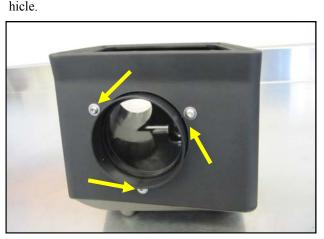
7. Mount the Filter Adapter (#5) to the Cold Air Box, as shown, using three  $1/4-20 \times 1/2$ " Button head Bolts (#16) and 1/4" Flat Washers (#17).
