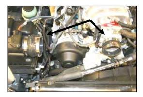
7. Install the small end of the urethane hump hose (#3) and the #56 hose clamp (#7) over the factory airbox. Install the #60 hose clamp (#8) onto the other side of the urethane hump hose. Next install the reducer coupler (#4), small side first, onto the throttle body with two #52 hose clamps (#9). Leave the clamps loose for now.
