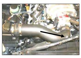
9. Install the MIT into the urethane hump hose first, and then into the reducing coupler. Adjust the MIT snugly against the throttle body, and tighten the 4 hose clamps. Next install the 1/4 - 20 button head bolt (#12) and 1/4" flat washer (#13) thru the Adel clamp and into the MIT to hold the air conditioning hose.
