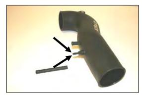
**8.** Install the 1/4" Barb x 1/8" NPT Fitting (#10) into the Airaid Modular Intake Tube (MIT) (#2) as shown. Now slide the 1/4" x 4" hose (#11) onto the barb fitting.
