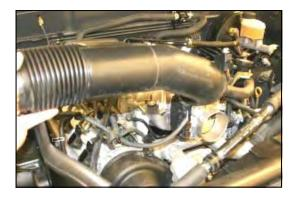
**4.** Remove the factory intake tube from the velicity
