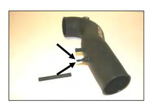
**8.** Install the 1/4" barb x 1/8" NPT fitting (#8) into the Airaid **M**odular **I**ntake **T**ube (**MIT**) (#2) as shown. Now slide the 1/4" x 4" hose (#9) onto the barb fitting.
