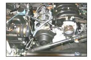
7. Install the urethane hump hose (#3) onto the factory airbox using two #60 hose clamps (#6). Next install the reducer coupler (#4), small side first, onto the throttle body using two #52 hose clamps (#7). Leave the clamps loose for now.
