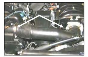
**3.** Loosen the hose clamps on the intake tube at the throttle body, and at the airbox.
