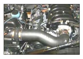
9. Install the MIT into the hump hose first, and then into the reducing coupler. Adjust the MIT snugly against the throttle body, and tighten the 4 hose clamps. Next install the 1/4 -  $20 \times 1/2$ " button head bolt (#10) and 1/4" flat washer (#11) thru the Adel clamp and into the MIT to hold the air conditioning hose.
