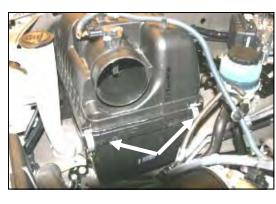
**5.** Unlatch the 4 clips on the factory airbox, and remove the lid.
