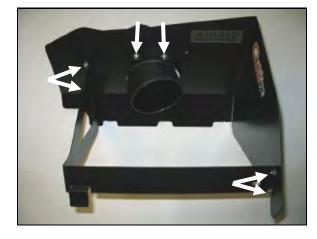
**5.** Assemble the Airaid Quick Fit Panels (#2, #3) using four 6-32 x 5/16" screws (#6), #6 flat washers (#7), and 6-32 keps nuts (#8). Next, install the air filter adapter (#4) using two  $\frac{1}{4}$ -20 x  $\frac{1}{2}$ " button head bolts (#9), and  $\frac{1}{4}$ " flat washers (#10).
