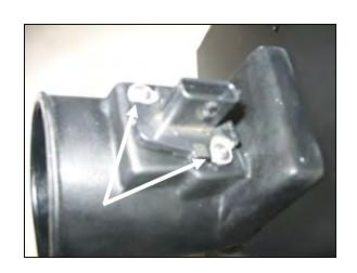
**6.** Using two 8-32 x  $\frac{1}{2}$ " SS button head screws (#11), reinstall the factory **MAF** sensor into the air filter adapter.
