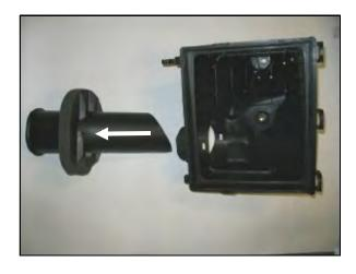
**4.** Remove the factory air box base from the vehicle. Using a flat blade screwdriver, unsnap and remove the factory tube from inside the air box base. Reinstall the factory air box base and the bolts into the vehicle, without the tube.
