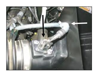
**9.** Reconnect the **MAF** sensor wiring harness to the sensor. Mount the factory wiring harness clip into the hole in the Airaid Quick Fit panel.
