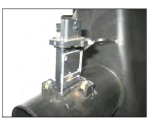
**3.** Using a Phillips head screwdriver, remove two screws and the **MAF** sensor from the factory air box lid. Save the sensor for reuse.
