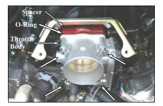
3. Install the O-Ring (#2) into the groove on the Poweraid Spacer (#1). Install the spacer between the intake manifold, and the throttle body with the O-Ring facing the throttle body. Insert four 6mm x 70mm Hex Bolts (#3), and 6mm Flat Washers (#4) through the throttle body, Poweraid Spacer, and into the intake manifold. Using a 10mm socket, tighten all 4 throttle body bolts evenly, to the manufacturer's specifications. **Do Not Over Tighten The Bolts!**
