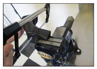
**6.** Firmly place the air scoop into a bench vice and cut along the line created in step **3** using a hack saw or equivalent.
