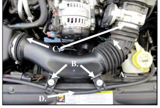
**2. A.**) Disconnect the air temp sensor in the factory intake. **B.**) Remove the two 6 mm bolts holding the intake tube to the fan Shroud. **C.**) Loosen the Clamps on both sides of the factory intake tube. **D.**) Unclip the coolant line from the intake tube and remove it from the vehicle.
