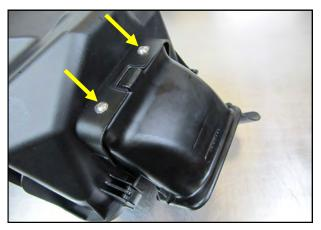
7. Re insert the modified air scoop into the air box and secure it using the # 8 Screws, Washers, and Nuts.
