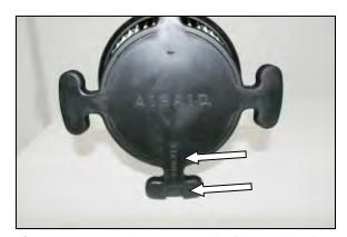
**4.** Locate the word "Down" on the filter, and notice that there is a notch in the urethane below it. It is important to locate this notch in the correct location in the bottom of the factory airbox.
