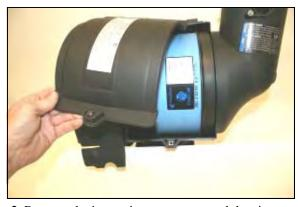
**2.** Remove the inspection cover to reveal the air filter.
