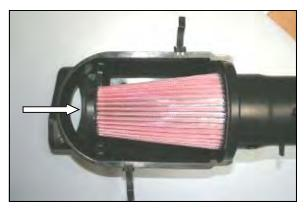
**3.** Insert the Airaid Premium Filter (#1) into the factory airbox.
