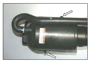
**1.** Unlatch the two factory clips on each side of the airbox and then remove the airbox lid.
