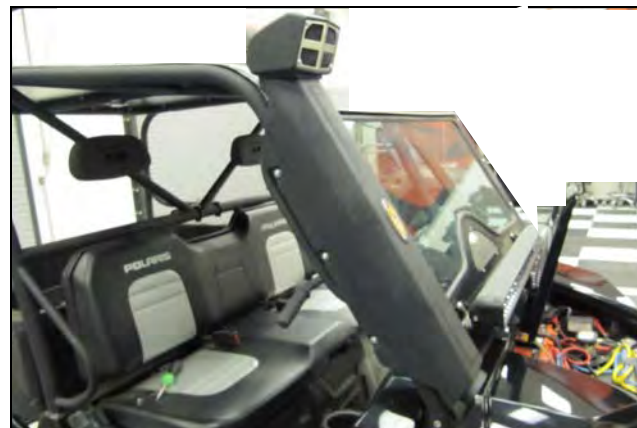
9. Outside view of properly placed Snorkel and clamps.
