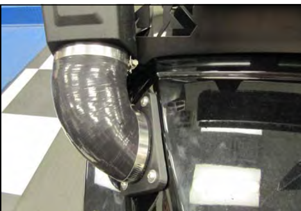
20. Install the trimmed Coupler with clamps (#9) onto the Snorkel tube and the Fender adapter. Tighten the Hose clamps and the three Snorkel Tube Clamps on the cage.
