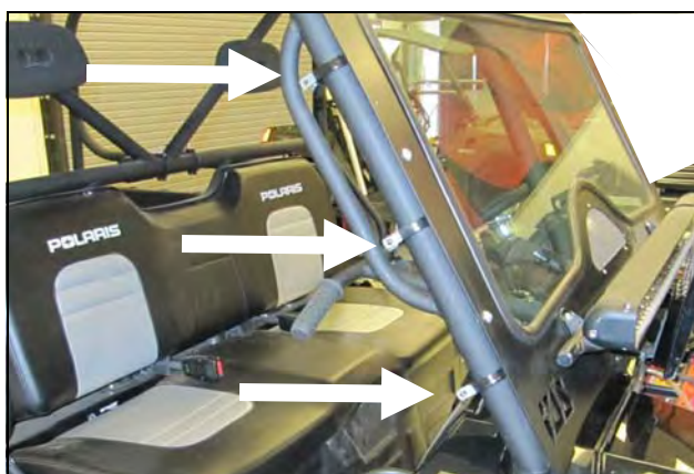
7. Preinstall the three Loop Clamps (#10) onto the right front A pillar of the cage.
