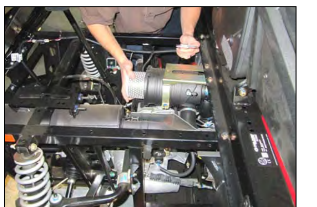
21. Tilt the bed back and install the Airaid Premium filter (#1).
