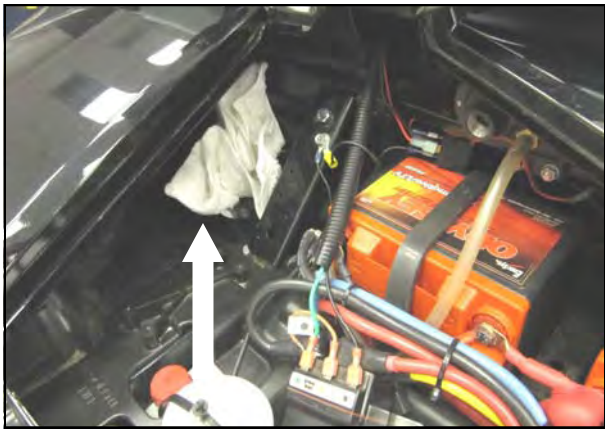
10. Place a shop towel inside of the factory inlet hose to prevent debris from entering.
