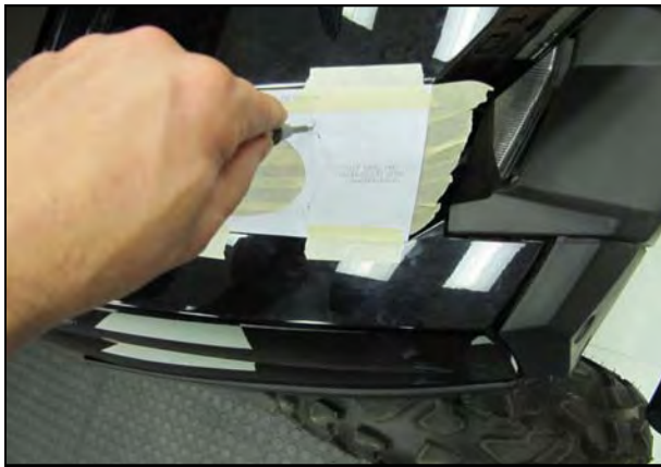
11. Prepare the right front fender for cutting by covering the entire area with masking tape. Cut out the Template and align all four edges against the radius of the fender. Tape down the template and mark the bolt holes with a center punch.
