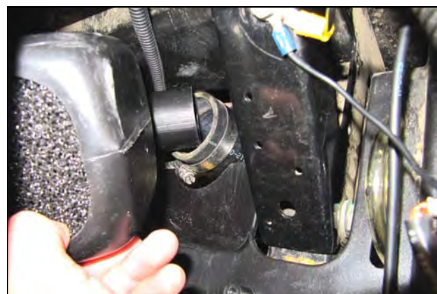
2. In the passenger side firewall area, locate the foam prefilter box and Loosen the hose clamp. Remove the prefilter box and set it aside.
