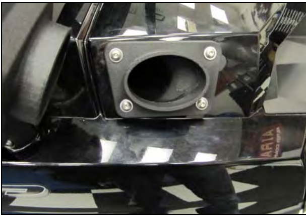
17. Mount the Adapter to the fender using Four 1/4-20 Button Head Bolts (#11), eight 1/4" Flat Washers (#13), and four 1/4-20 Locknuts (#12). Tighten the factory air inlet hose clamp.
