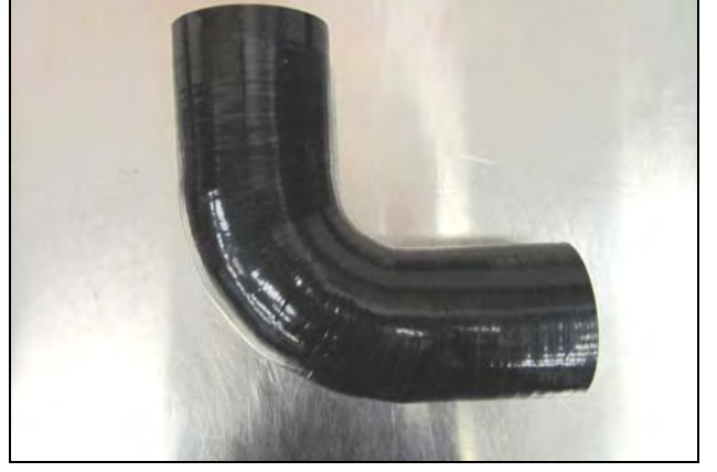
18. To accommodate many cage variations, this kit is supplied with an oversized Tube to Adapter coupler (#6). Determine the required trim lengths for your particular application and mark the coupler with a permanent marker.
