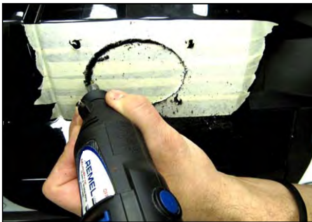
14. Using a Dremel type rotary tool and a 1/8" drill bit, plunge into the inner oval at medium speed and cut along the line until the center falls out. Remove the tape.
