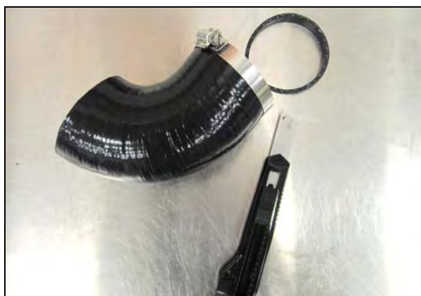
19. Once you have your coupler length marked, slide a hose clamp (#9) onto the coupler and tighten the clamp along the mark. Use the hose clamp as a guide to trim the coupler to length with a sharp utility knife.
