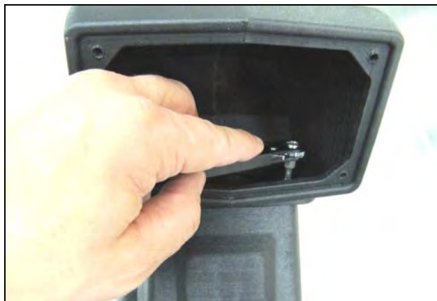
3. Mount the Snorkel Inlet to the Snorkel Tube (#1), using the four Torx screws (#14) and a 90deg. Low Profile Ratcheting Screwdriver.
