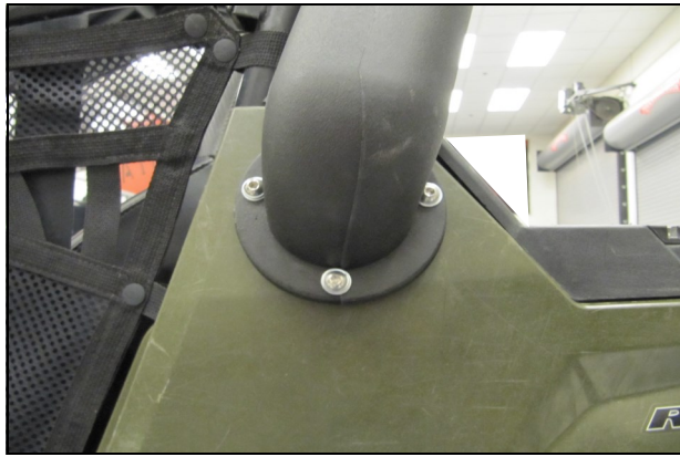
12. Replace the Threaded Studs, one at a time, with the remaining 1/4-20 x 1" Button Head Bolts and 1/4" Washers from the previous step. Make all three Bolts final tight.
