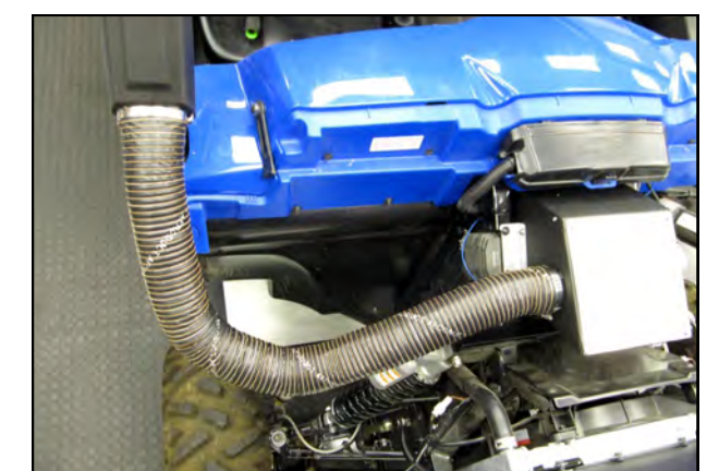
36. Full view of Duct routing.
