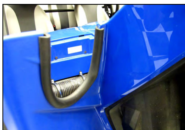
38. Slide the 10 inch Edge Trim (#25) over the cut out on the Hood.
