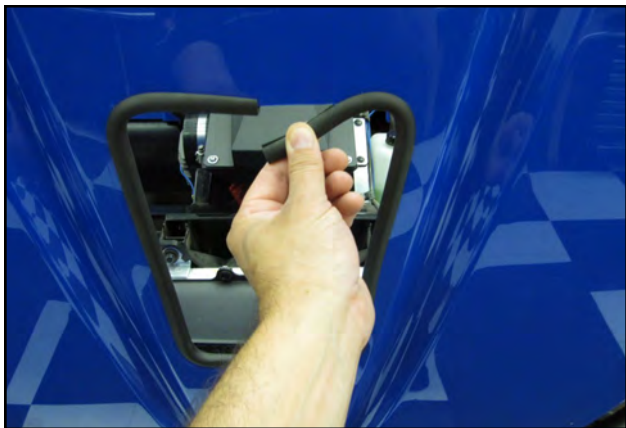
16. Install the 36" Edge Trim (#21) onto the hood, trim to fit.
