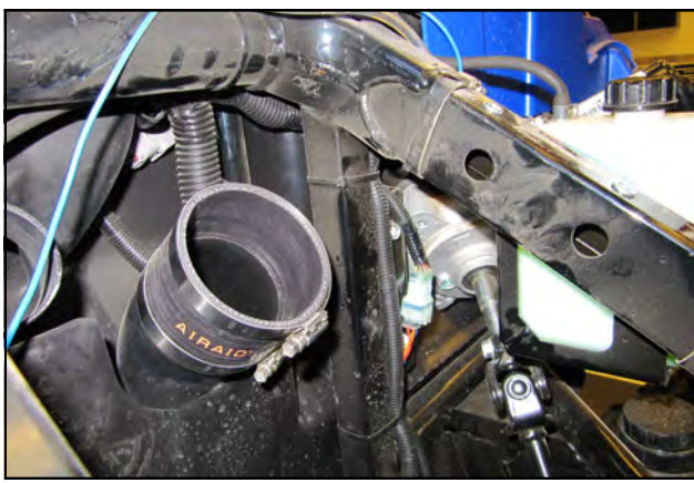
10. Install the Silicone Coupler (#8) and Two #48 Hose Clamps (#18) onto the factory intake tube. Leave the Clamps loose for now.
