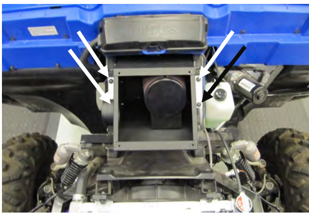
11. Insert the Airbox outlet into the Silicone coupler and tighten the Clamps. Mount the Airbox to the vehicle by reusing the factory hardware from step 1. STOP! If you plan to install the Snorkel kit, proceed to step 23.
