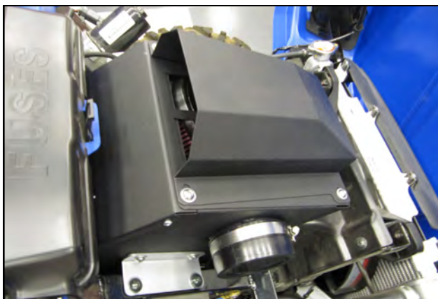
19. Install the Hood Scoop onto the Airbox Assembly using the four sets of 1/4-20 x 1/2" Button Head Bolts (#20) and 1/4" Flat Washers (#21). Leave the bolts loose for now to allow for final adjustment.
