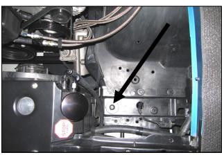
**3. Driver Side** - Remove the inner fender bolt and set it aside. It will be re used in step #7.
