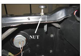
**4.** Install the L bracket (#5) under the core support .Use the 5/16 Flange nut (#7) to secure it to the lower portion of the hood stop.
