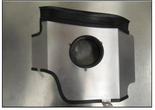
**2.** Install the Weather Strip (# 4) across the top edge of the Air dam, and the Edge Trim (#6) along the bottom edge. Trim pieces to desired length.
