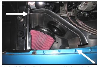
**6.** Carefully install Air Dam assembly in to the inner fender area. **Note-**The outermost edges will be underneath the core support and the fender when installed properly.
