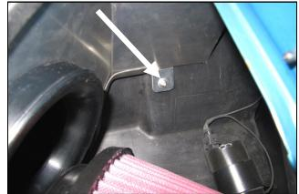
**9.** The third mounting point will need to be drilled into the inner fender. Secure the Air Dam tab using one 1/4-20 Button Head Bolt, one 1/4" Flat Washer topside, and the Fender Washer (#10) and the last 1/4-20 Nylock nut from below.
