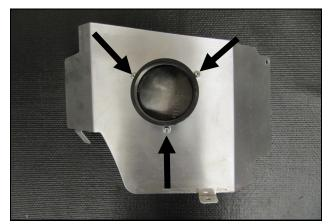
1. Remove the protective film from the sheet metal. Install the Filter Adapter (#3) onto the Air Dam (#2) using three sets of 1/4-20 Button Head Bolts (#8), and 1/4" Flat Washers (#9).
