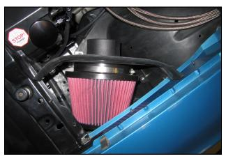
**10.** Install the Airaid premium onto the Filter adapter and tighten the clamp..
