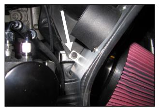
**7.** Align the Aid Dam tab with the factory bolt hole from step #3 and secure it by reusing the factory bolt.
