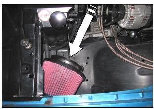
**5.** Tuck the Airaid premium Filter (#1) into the inner fender.
