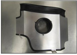
**2.** Install the Weather Strip (# 4) across the top edge of the Air dam, and the Edge Trim (#6) along the bottom edge. Trim pieces to desired length.
