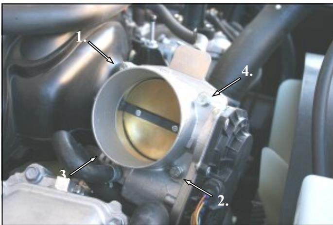
5. Reinstall the factory bolts and tighten them in a cross pattern to the manufacturer's specifications. Before starting the engine, open and close the throttlebody to make sure there are no obstructions.
