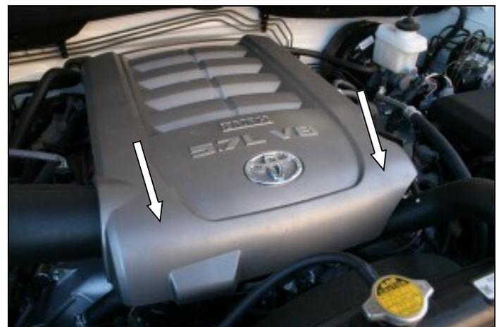
6. Reinstall the air intake tube and reconnect the hoses and electrical connectors. Tighten all hose clamps. Reinstall the beauty cover.
