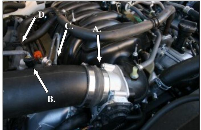
2. **A.)** Loosen two hose clamps, one at the air box, and one at the throttlebody. **B.)** Squeeze the tab on the electrical connector and disconnect it from the Mass Air Sensor. **C.)** Disconnect the 1/8" vacuum line from the air intake tube. **D.)** Disconnect the crankcase breather hose from the intake tube. Remove the air intake tube from the vehicle.
