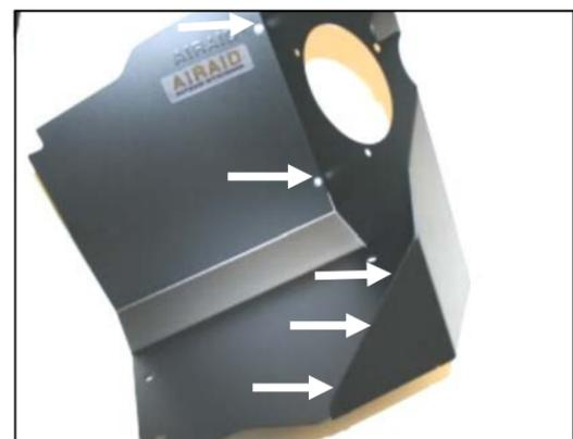
**5.** Assemble the Airaid Cool Air Dam panels (#2, #3) using five 6-32 x 5/16" screws (#9), #6 flat washers (#10) and 6/32 keps nuts (#11). Apply the Airaid Foil Decal onto the Panel as shown.
