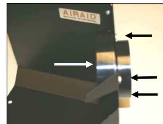
**6.** Using three 1/4-20 x 5/8" hex bolts (#12) and 1/4" flat washers (#13), install the filter adapter (#4) onto the Airaid Cool Air Dam.
