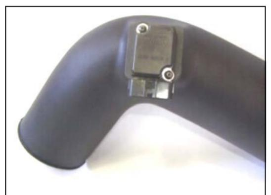
**9.** Using two 8-32 x 1/2" button head screws (#15) install the factory M.A.F. sensor in the Airaid intake tube (#5) **DO NOT USE THE FACTORY SCREWS!** (Note: Sensor must be installed in the direction shown in the picture, with steel washers between it and the tube.)
