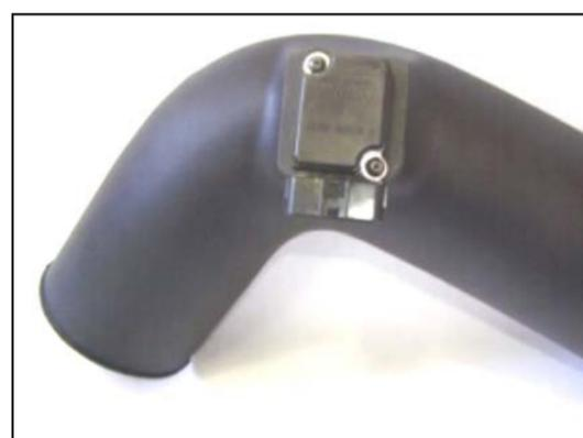
**9.** Using two 8-32 x 1/2" button head screws (#15) install the factory M.A.F. sensor in the Airaid intake tube (#5) **DO NOT USE THE FACTORY SCREWS!** (*Note: Sensor must be installed in the direction shown in the picture, with steel washers between it and the tube.*)
