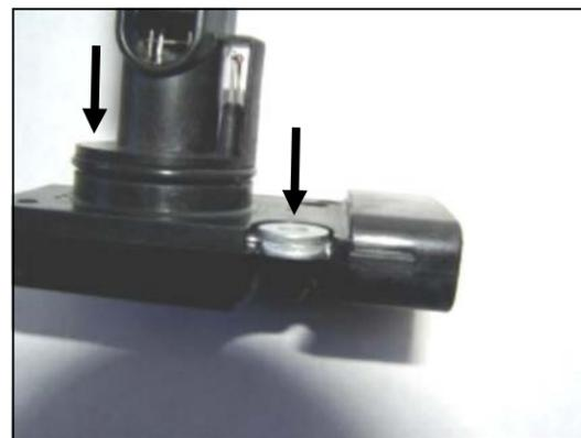
**8.** Place two steel washers (#16) into the recessed portions of the MAF sensor mounting holes.
