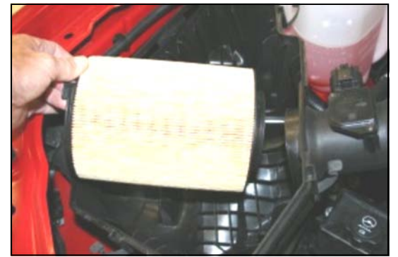
3. Remove the factory air filter, and set it aside.
