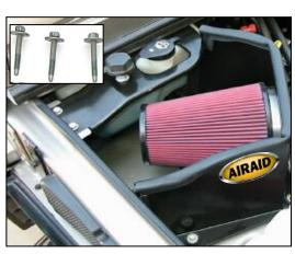
**9.** Position the Airaid system over the three factory mounting points & secure with the three saved factory bolts removed in step #4.Apply the Airaid Foil Decal onto the Panel as shown.
