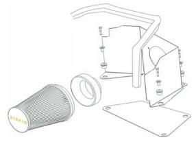
**6.** Align Cool Air Dam panels (#2, #3) & fasten together with saved grommets and bushings from step #4. Install the filter adapter (#4) using the 3 provided button head bolts (#9) and washers (#10).
