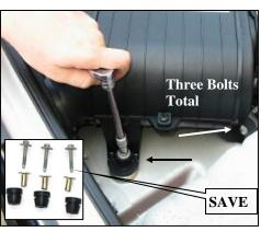
**4.** Remove the three factory air box hold down bolts, bushings, and grommets. Save them for the Airaid installation.
