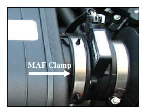
**3.** Loosen the Mass Air Flow sensor hose clamp. Remove the MAF sensor from the factory air box and temporarily set it aside. Use caution to retain the factory coupler & hose clamp on the MAF.
