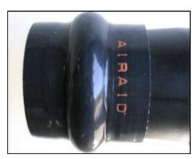
**12.** Install the provided urethane hump hose (#7) onto the Airaid **M**odular **I**ntake **T**ube (**MIT**) (#5) with the 2 supplied #60 hose clamps (#11). **Note:** Leave hose clamps loose until final assembly.
